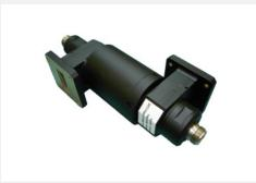
Our custom designed waveguide rotary joints can be offered as pressurised and non-pressurised, single, or multi-channel, with a selection of waveguide or coaxial connections and I-type, L-type, or U-type geometrical layout. Sizes are offered from WR137 to WR28 with any combination of interfaces required by the customer.
