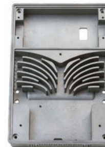
Cast example of thick and thin wall sections
