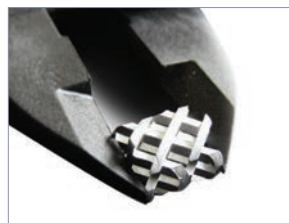
This casting is a maze of holes. Its perfect surface is due to easy mould removal.
